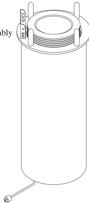
HEIGHT FROM MOUNTING SURFACE TO BOTTOM OF UNIT IS 25" / 635 mm.
